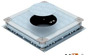
Underfloor accessory socket for screed-covered underfloor installation ducts with sheet steel side walls. To mount installation units of the selected nominal size. Height can be infinitely adjusted to the nominal screed height (rapid adjustment possible) and the screed can be worked flush to the screed scraping edge. With noise decoupling option after screed laying and can be used with system accessories, also for heavy-duty application.
