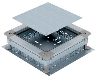
Underfloor junction and branch box for 7 installation pipes on each side (M20 or M32) with sheet steel side walls. To mount installation units in the mounting lid (to be ordered separately). Height can be infinitely adjusted to the nominal screed height (rapid adjustment possible) and the screed can be worked flush to the screed scraping edge. With noise decoupling option after screed laying and can be used with system accessories, also for heavy-duty application.
