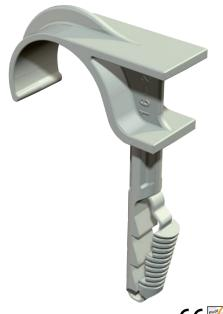
These push-fit clips are used when installing cables and pipes on walls and ceilings and when running flexible pipes on concrete and in the screed. The single push-fit clips can be used instead of nail clips in concrete and aerated concrete. The advantage of the push-fit clips is that they only have to be pushed into the drilled hole. Anchors and bolts are not needed.
