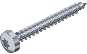
Hardened steel, electrogalvanised and Hostaflon-coated. Pan head with T bit (Allen head), sizes  $\emptyset$ 3 mm T10, Ø 3.5 mm T15, Ø 4 and 4.5 mm T20, Ø 5 mm T25.
