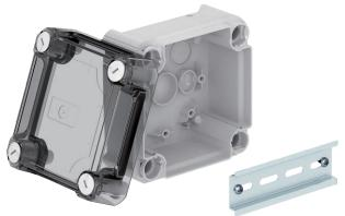
Closed junction box for the connection of cables and lines indoors and in protected outdoor areas. Square design without entries. Suitable for wall and ceiling mounting and on mounting panels. With the option to fasten inside and to mount via the corner domes. High, transparent cover with quick lock, sealable. Made from halogen-free materials. With hat profile rail.
